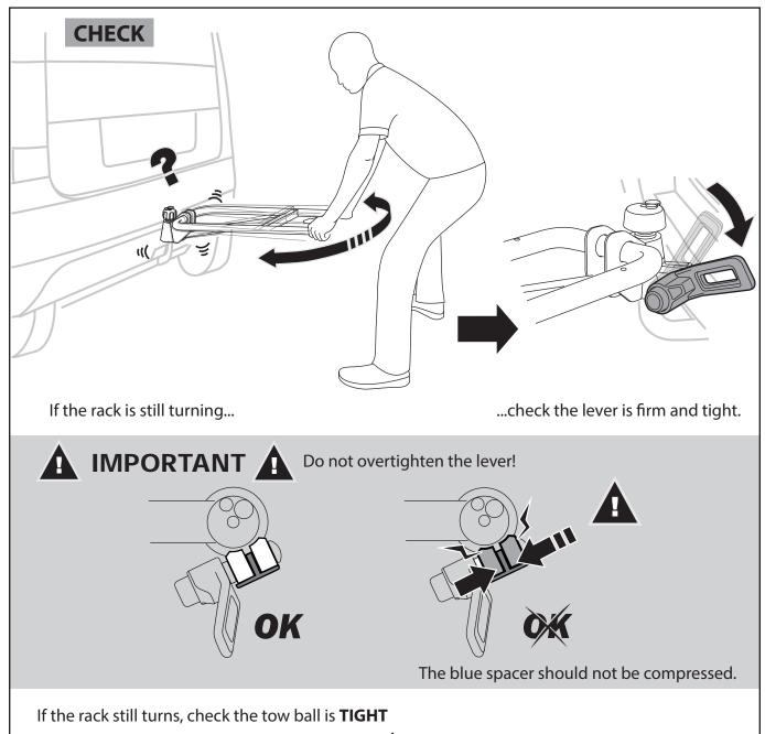
Try turning the rack while looking underneath at the towball base and nut, if the ball is loose it will visibly turn with the rack. Tighten the towball until the rack stops turning.
